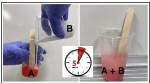
4. Pour the silicone mixture into the mold. Only fill the mold up to the ledges as seen below. Be sure to not overfill the mold since a second silicone mixture will be added later. This layer will take approximately 12 hours to cure at room temperature.
