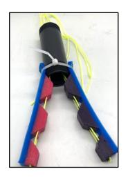
10. Feel free to combine your actuator with another group's actuator to create a claw. Secure the ends along the outside of a tube with a zip-tie.
